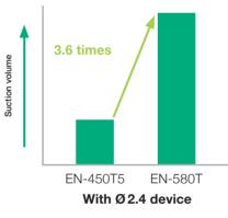
The 3.2 mm working channel provides greater suction performance than conventional models. (According to Fujifilm data)
